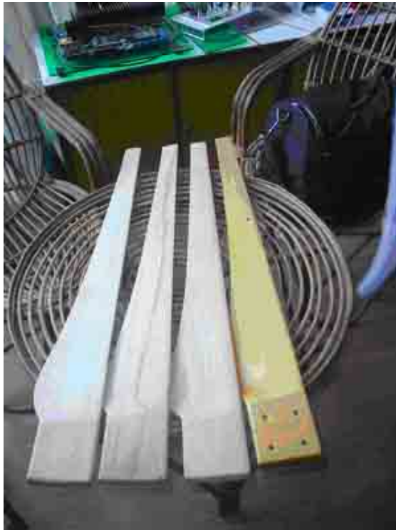
Nepali handmade blades for wind turbines
