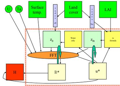
Fig. 1 Microscale model based on Hasager and Jensen (1999) but with new inclusion of land cover type and leaf area index maps for direct calculation of the aggregated scalar roughness,  $z_0$  (Hasager et al. 2002).
