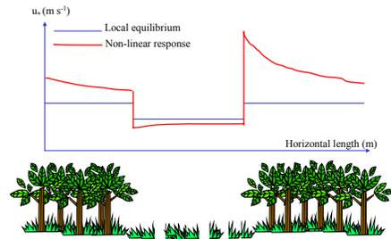
Fig. 2 The friction velocity ( $u_*$ ) varies downstream as a function of local roughness and patch size. The equilibrium values (for very large patches) and the real non-linear behaviour is shown.
