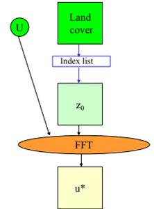
The non-linear variations of friction velocity ( $u_*$ ) is modelled in a horizontal 2-dim domain for arbitrary roughness variations in real terrain by a microscale surface-flux aggregation model. The effective roughness is calculated per HIRLAM grid cell (for references see below)
