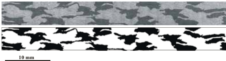
Fig. 4. Hybrid glass/carbon fibre composite with \beta = 0.28 and \gamma = 0.35 (CXG-07): original grayscale image (top), and resulting binary image (bottom).
