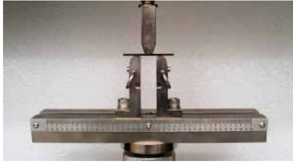
Fig. 4. Three-point flexural fixture.
