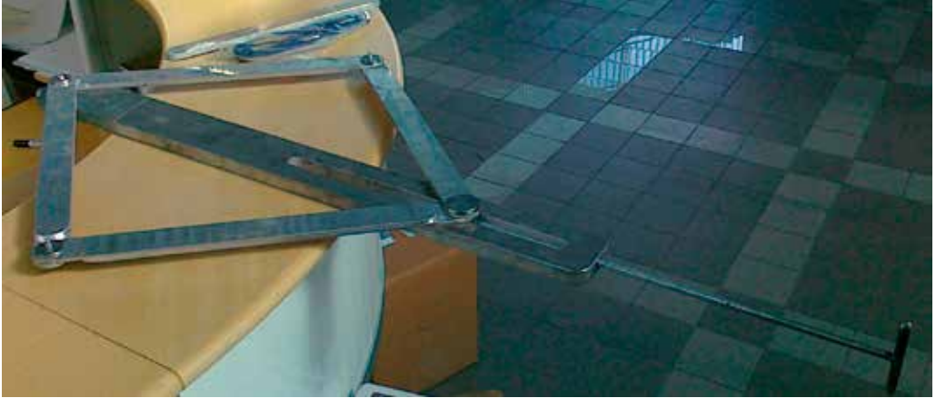
Fig 1: The delivered Trellis frame for shearing of multiple ply lay ups. The four moving arms are mounted on a support frame with a tensioning screw for controlling the shear angle of the plies. Above the Trellis frame one welding tong and one clamping bar is visible.
