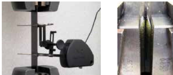
Fig. 3. Tensile test fixture; left: a sample gripped and mounted with a 50 mm extensometer, right: a sample end tabbed to prevent damage at grip areas.
