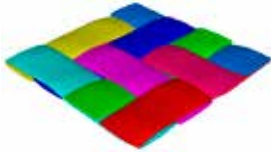
Fig. 14. Unit cell model of TW in TexGen.
